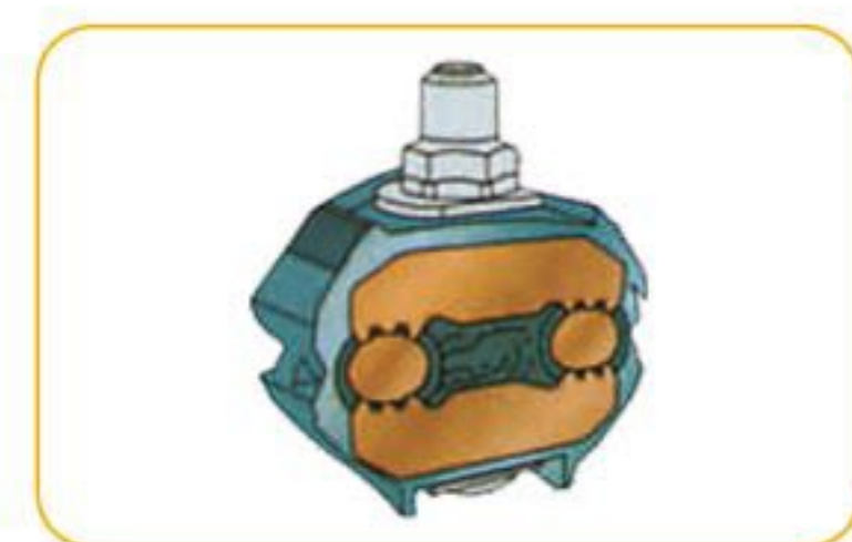
Section diagram of piercing effect
